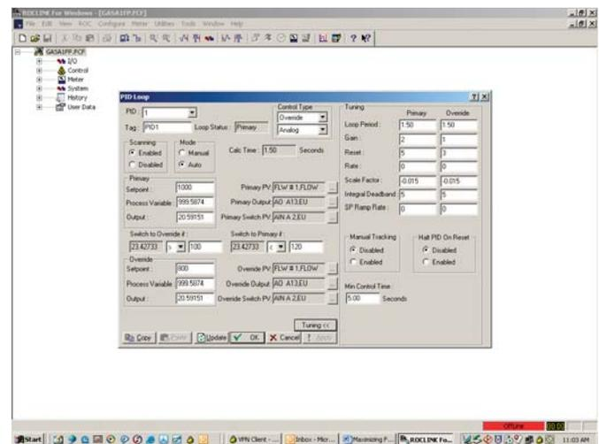
to allow assigning process variables, outputs, and gain settings. In the oil and gas production environment, this type of control can be configured for either analog output to a valve current to pressure transducer (I/P) or digital, with a single discrete output for valve opening and one for valve closing. Both methods have their advantages, depending upon power available at the site, air or gas source for valve diaphragms, speed of response, and cost.
